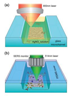
Scheme 1 Sketch of femtosecond laser fabrication of the silver SERS substrate inside a microfluidic channel (a), and the application of this SERS monitor for target molecule detection at visible light (514.5 nm) excitation (b).
