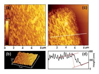
**Fig. 3** AFM characterization of the silver SERS substrate. (a) The surface of one silver substrate; (b) 3D view of the silver substrate; (c) one corner of the silver substrate and (d) the height profile along the white line.
