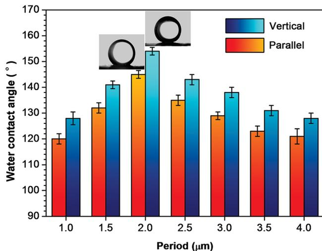
**Figure 3.** Dependence of the CA in both vertical and parallel directions of the grating structure on the grating periods from 1.0 to 4.0  $\mu\text{m}$ . The insets are the photographs of a water droplet on superhydrophobic graphene film with a period of 2.0  $\mu\text{m}$  viewed from vertical and parallel direction.
