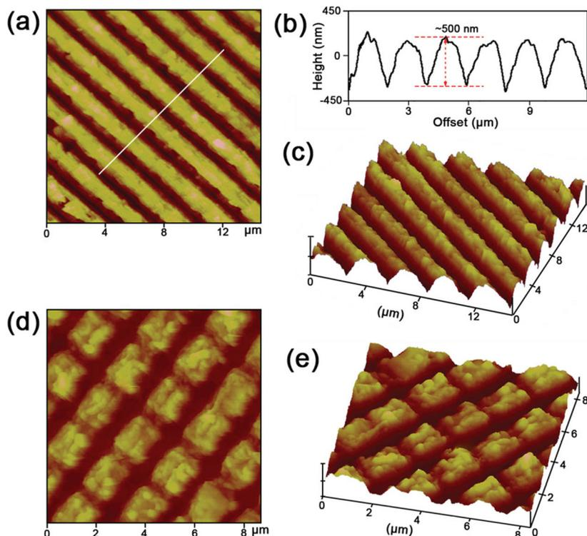
**Figure 5.** a–c) AFM image of superhydrophobic graphene films with 1D grating-like structures fabricated by TBLI. b) Height profile of the surface along the white line in (a). d,e) AFM image of superhydrophobic graphene films with 2D grating-like structures fabricated by dual TBLI treatment with 90° rotation.
