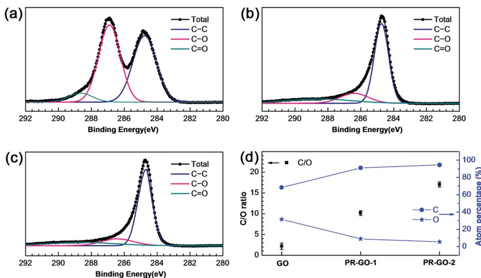
**Figure 6.** C1s XPS spectra of pristine a) GO and RGO films prepared by b) TBLI and c) dual TBLI treatment with 90° rotation. d) C/O atom ratios and the atom contents (C, O) of GO, and RGO films prepared by TBLI and dual TBLI treatment with 90° rotation.
