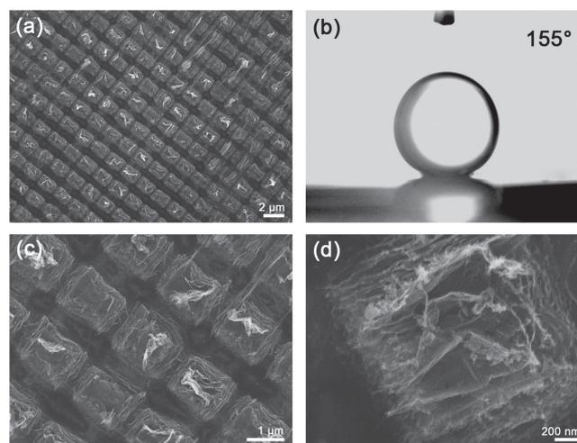
**Figure 4.** a) SEM images of superhydrophobic graphene film with 2D grating-like structures. The period is 2.0  $\mu\text{m}$ . b) Photograph of a water droplet on its surface, the CA is measured to be  $\approx 155^\circ$ . c,d) Magnified SEM images of 2D grating-like structures.
