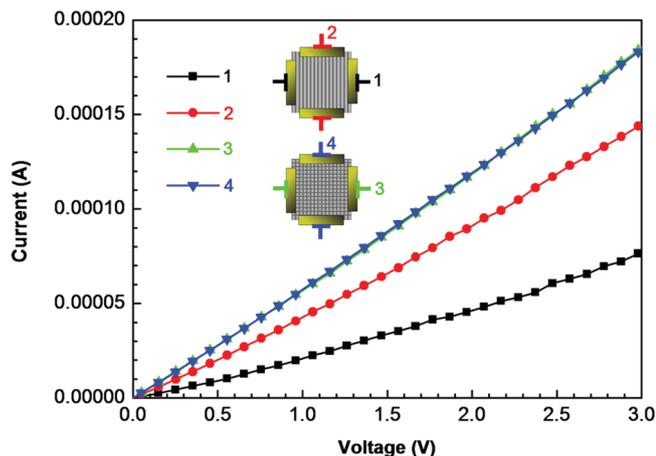
**Figure 7.**  $I$ - $V$  curves of RGO films with 1D and 2D grating-like structures measured on both vertical and parallel directions. The insets are schematic illustrations of the  $I$ - $V$  measurements.
