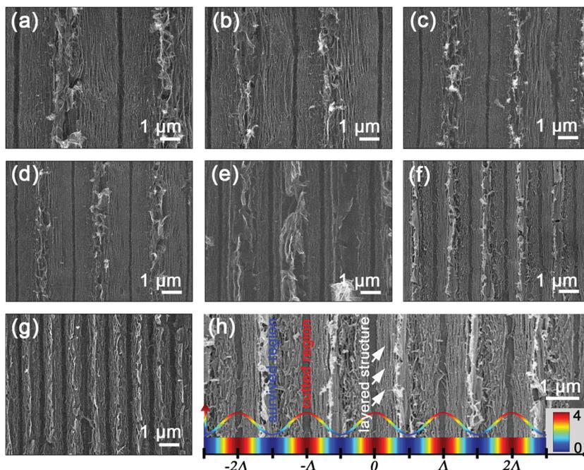
**Figure 2.** SEM images of TELI treated graphene films with different periods, a) 4  $\mu\text{m}$ , b) 3.5  $\mu\text{m}$ , c) 3  $\mu\text{m}$ , d) 2.5  $\mu\text{m}$ , e) 2  $\mu\text{m}$ , f) 1.5  $\mu\text{m}$ , g) 1  $\mu\text{m}$ . h) SEM image and the contrastive laser intensity distribution.
