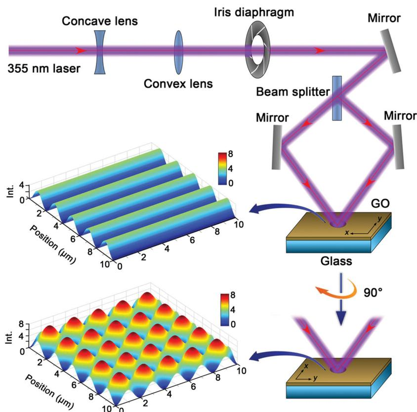
**Figure 1.** Schematic illustration of the fabrication of superhydrophobic graphene films by TBLI and dual TBLI treatment with 90° rotation. The insets are laser intensity distributions of TBLI and dual TBLI treatment with 90° rotation, which are calculated by Matlab.
