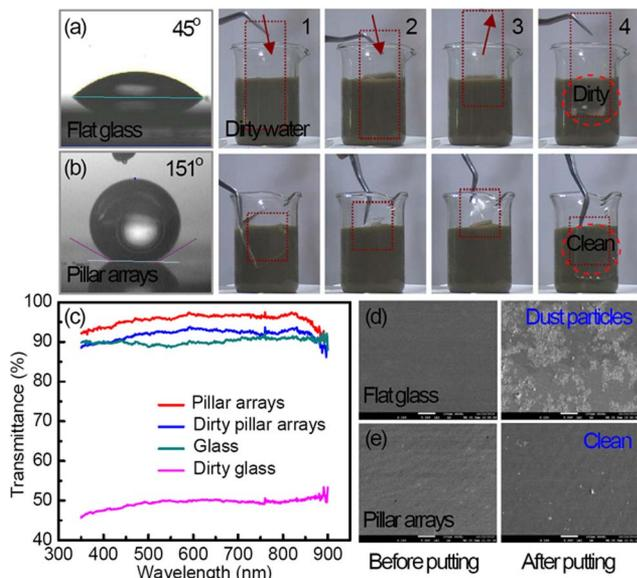
Fig. 4. (Color online) Self-cleaning superhydrophobic ability of the nanopillar arrays. (a) and (b) The wetting property and antidust ability of the flat surface and nanopillar arrays. (c) The optical transmittance before and after being immersed into dirty water. (d) and (e) Comparison of the flat glass and pillar arrays characterized by the SEM image.
