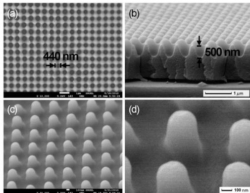
Fig. 2. Antireflective nanopillar arrays prepared by low-cost imprint lithography. (a) Top-view from the SEM of the hole template. (b) Cross-sectional SEM image of the template. (c) and (d)  $45^\circ$  tilted-view of the SEM and locally magnified image of the regular nanopillar arrays.
