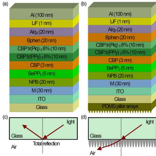
Fig. 1. (Color online) External quantum efficiency enhancement of white OLEDs by antireflective films. (a) and (b) The reference OLEDs structure and the OLEDs with antireflective films. (c) and (d) The light outcoupling mechanism.
