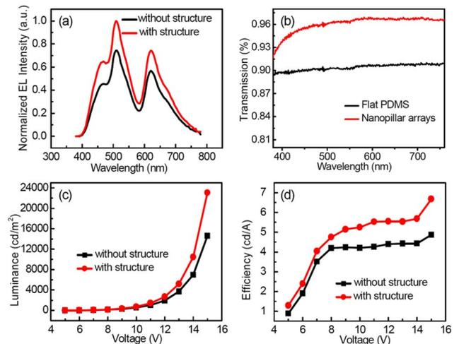
Fig. 3. (Color online) (a) Enhanced EL intensity in the normal direction of the OLEDs by the antireflective films. (b) The optical transmittance spectra of the flat PDMS surface and nanopillar arrays. (c) and (d) Luminance and current efficiency characteristics of the OLEDs with and without antireflective films as a function of current density.
