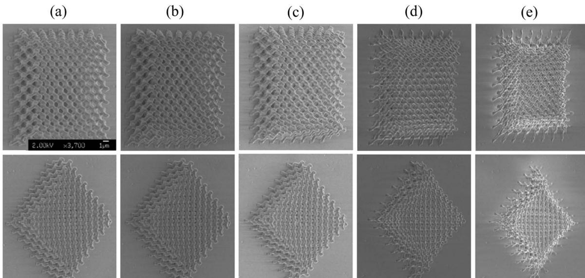
FIG. 3. SEM images of diamond-lattice PhCs heated under different temperatures for 30 min: (a) as fabricated at RT, (b) 150  $^{\circ}\text{C}$ , (c) 200  $^{\circ}\text{C}$ , (d) 250  $^{\circ}\text{C}$ , and (e) 300  $^{\circ}\text{C}$ .
