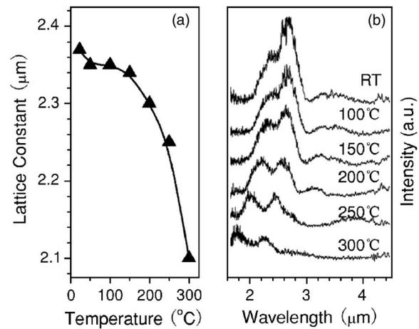
FIG. 4. (a) The treatment temperature-dependent lattice constants of the heated PhC. (b) Reflection spectra of the PhC structures treated under different temperatures.
