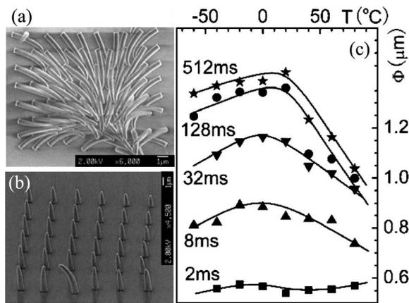
FIG. 2. Spatial resolution investigation by means of voxel formation. (a) Long voxels and (b) approximately half-truncated voxels produced by the ascending scan approach. The applied laser pulse energy is 8 nJ. (c) Lateral voxel sizes under varied temperatures. Each point is obtained by averaging data from six identical experiments.
