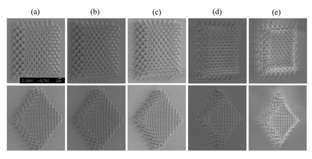
FIG. 3. SEM images of diamond-lattice PhCs heated under different temperatures for 30 min: (a) as fabricated at RT, (b) 150 °C, (c) 200 °C, (d) 250 °C, and (e) 300 °C. Downloaded 20 May 2009 to 59.72.114.11. Redistribution subject to AIP license or copyright; see http://apl.aip.org/apl/copyright.jsp
