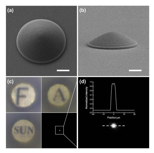
Figure 2. (a) SEM image of hyperbolic microlens from PEG-DA hydrogel with a radius of  $10 \,\mu m$  and height of  $5 \,\mu m$ . (b) Side-view image of the hyperbolic microlens. (c) Focusing test and imaging test of PEG-DA microlens in air. (d) Normalized light intensity distribution along the dotted line. Scale bar:  $5 \,\mu m$ .
