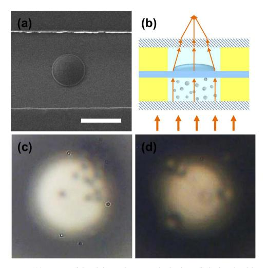
Figure 4. (a) SEM image of a hyperbolic microlens integrated within the optofluidic channel. Scale bar:  $50\,\mu m$ . (b) Schematic of the focusing characteristic resulting from the PEG-DA microlens in the integrated twin optofluidic and microfluidic channels. (c,d) Images of polystyrene spheres and HUVEC formed by a microlens using the twin optofluidic and microfluidic channels.
