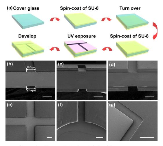
**Figure 1.** (a) Process flow of the twin optofluidic and microfluidic channels fabrication. Cross-section SEM images of twin microchannels with depths of  $15\,\mu\text{m}$  (b),  $33\,\mu\text{m}$  (c) and  $45\,\mu\text{m}$  (d), respectively. (e–g) SEM images of microchannels with different widths of  $200\,\mu\text{m}$  (e),  $100\,\mu\text{m}$  (f) and  $50\,\mu\text{m}$  (g), as well as various shapes: cross-shaped (e), spherical (f), orthogonal (g). Scale bar:  $100\,\mu\text{m}$ .
