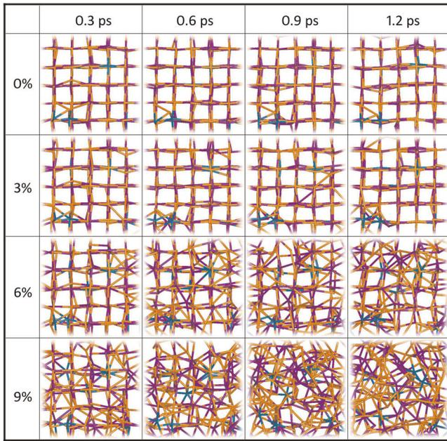
**Fig. 1 Structural evolution of Sc-Sb-Te upon optical excitation.** Structures (in a bond stick model) of rocksalt Sc-Sb-Te under optical excitation of valence electrons from 0 to 9% (rows) at 0.3, 0.6, 0.9, and 1.2 ps (columns), respectively. Color coding: Cyan for Sc, purple for Sb, and orange for Te.
