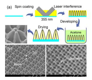
FIG. 1. (Color online) Fabrication of regular flowerlike arrays by combinative use of multibeam interference patterning and capillary force selforganization. (a) The fabrication process: spin coating, laser beam interference, development, and drying. (b) and (c) are 45°-tilted and bird's eye view SEM images of the array.
