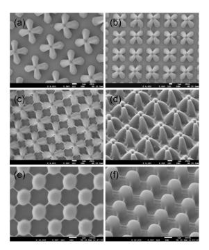
FIG. 2. Complex periodic nanostructures under varied exposure conditions. (a)–(c) are top-view SEM images of nanoflowers formed under exposure of 3, 4, and 5 s, respectively. (d) 45°-tilted SEM image of the 5 s exposed nanoflower array. (e) and (f) are top and tilted view SEM images of complex network arrays produced from 1.5  $\mu$ m thick sample by long exposure of 8 s.
