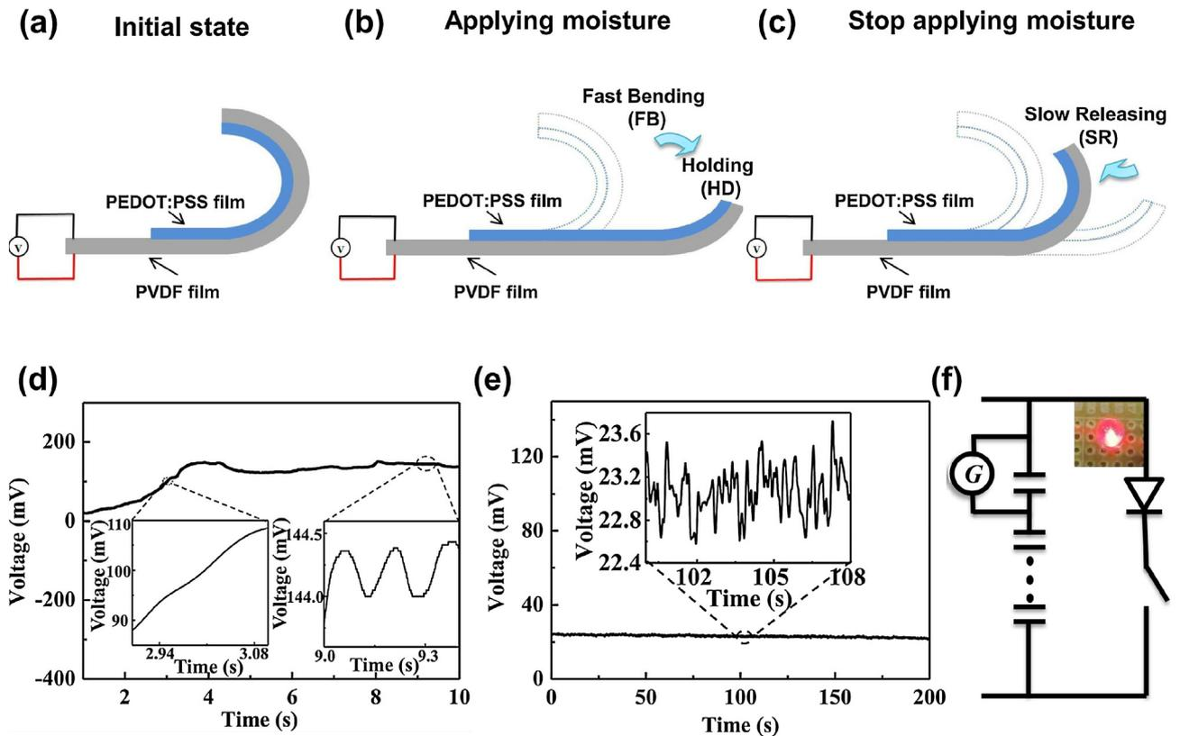
**Fig. 4.** (a)–(c) Schematic illustration of the PEDOT: PSS/PVDF double-layered generator produce a stable DC output voltage. (d) and (e) The output electrical signal generated by the generator during the humidification process (d) and dehumidification process (e), respectively. The inset is an enlarged view of the region of the curve. (f) The equivalent circuit diagram of the PEDOT: PSS/PVDF double-layered generator charges the capacitor to turn on the LED. The inset is the illuminated LED.
