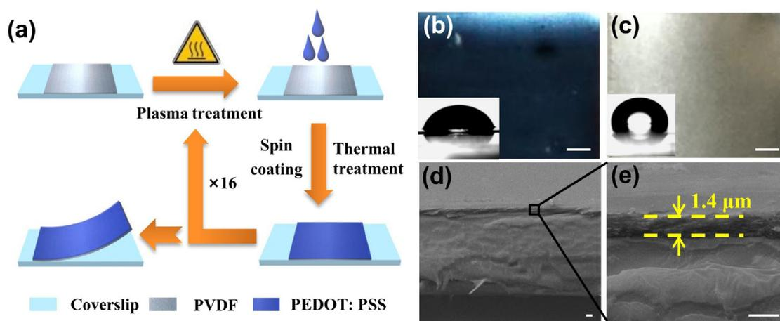
**Fig. 1.** (a) Schematic illustration of the fabrication process of the PEDOT: PSS/PVDF double-layered actuator. (b) and (c) Photographs of the PEDOT: PSS/PVDF double-layered actuator viewed from the PEDOT: PSS side (b) and the PVDF side (c), respectively (scale bar represents 1 mm). The insets show water droplet contact angles of both sides. (d) and (e) SEM images of a cross section of the PEDOT: PSS/PVDF double-layered actuator (scale bar represents 2  $\mu\text{m}$ ).
