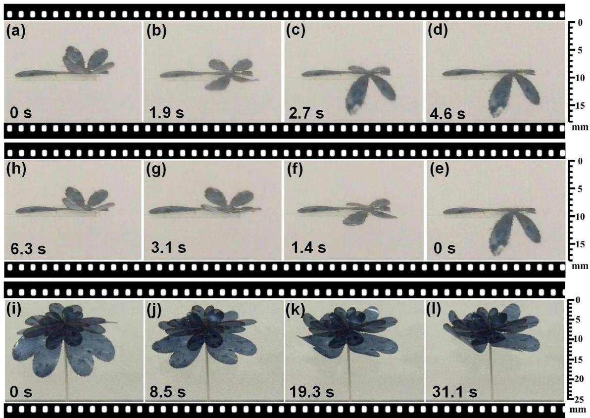
**Fig. 3.** (a)–(h) Biomimetic dragonflies with moisture response fabricated by PEDOT: PSS/PVDF composite film. (i)–(l) Three-layer-structure of flower assembled from three different sized four-petal flowers. The different components of the three-layer-structure of flower produce different responses under the same external stimuli.
