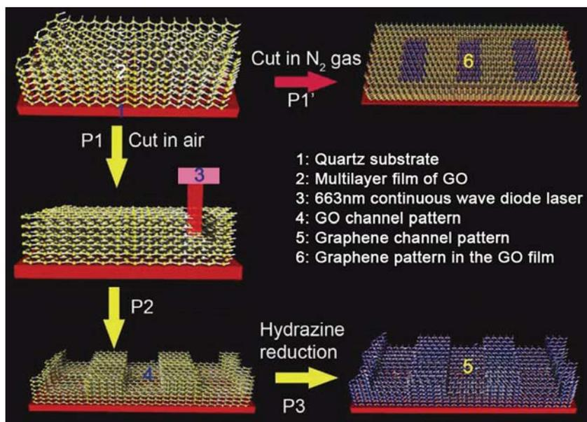
**Figure 5.** Schematic illustration of the cutting and patterning of GO nanosheets by a focused laser beam. For simplicity of the illustration, the hydroxyl, ether, and carboxylic groups of GO were omitted, and yellow represents GO and blue represents graphene. Reproduced with permission.<sup>[122]</sup> Copyright 2010, John Wiley and Sons.
