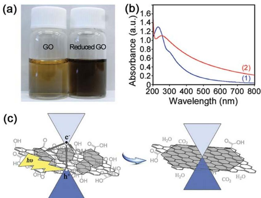
**Figure 4.** a) Photographs of GO and RGO solution; b) UV-vis spectra of nanosheet suspensions of (1) GO and (2) RGO prepared by photoreduction in H<sub>2</sub> for 2 h. Reproduced with permission.<sup>[115]</sup> Copyright 2010, American Chemical Society. c) Schematic illustration of the photochemical reduction mechanism of GO to RGO. Reproduced with permission.<sup>[84]</sup> Copyright 2012, John Wiley and Sons.
