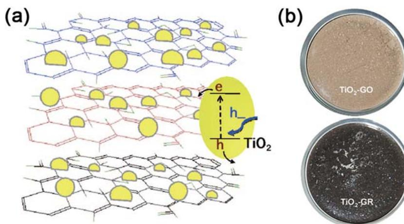
**Figure 3.** a) Schematic illustration of TiO<sub>2</sub>-assisted photoreduction of GO under UV excitation; b) photographs of TiO<sub>2</sub>-GO composite before and after reduction. Reproduced with permission.<sup>[69]</sup> Copyright 2008, American Chemical Society.
