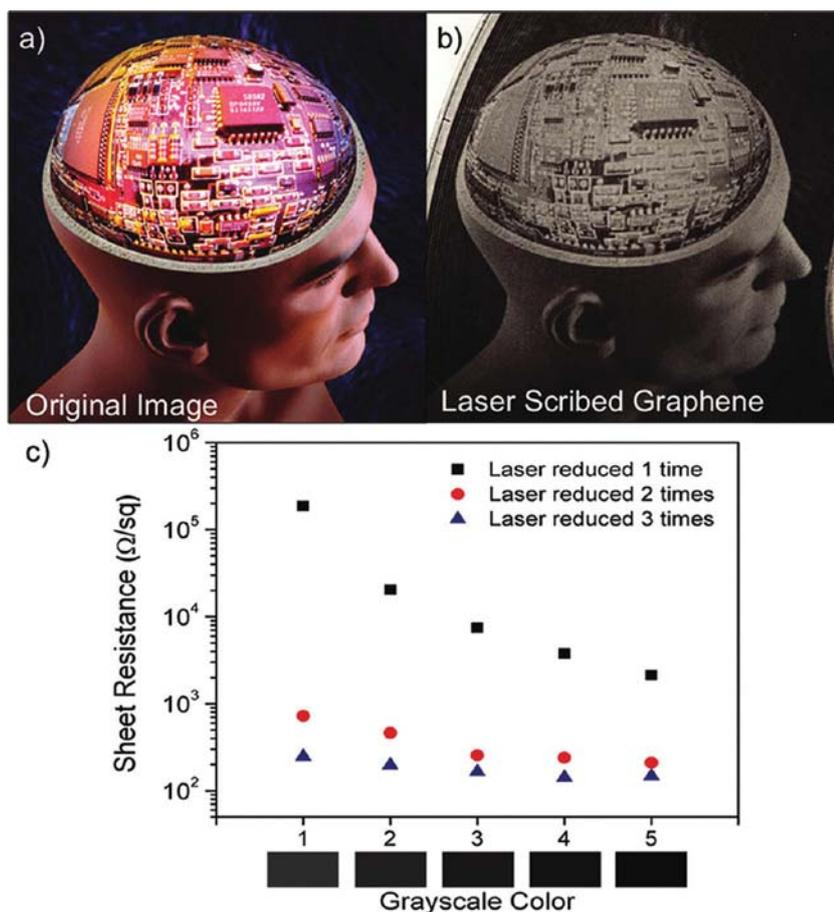
**Figure 8.** a) A complex colored image of a man's head filled with circuits; b) the same image reproduced on a GO film. The difference in color corresponds to a change in electrical properties. c) A correlation between laser intensity and sheet resistance. Reproduced with permission.<sup>[126]</sup> Copyright 2012, American Chemical Society.
