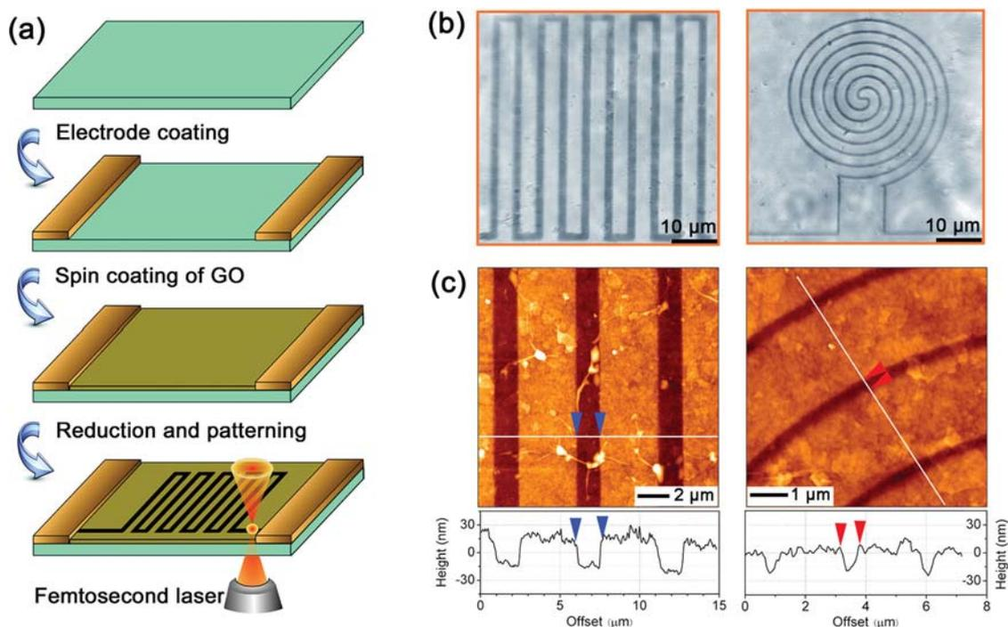
**Figure 7.** a) Schematic illustration of the FsLDW reduction and patterning of GO; b) optical microscopic images of different micropatterns; c) AFM image of the detail of micropatterns, the bottom two images show the profile of the micropatterns. Reproduced with permission.<sup>[87]</sup> Copyright 2010, Elsevier.
