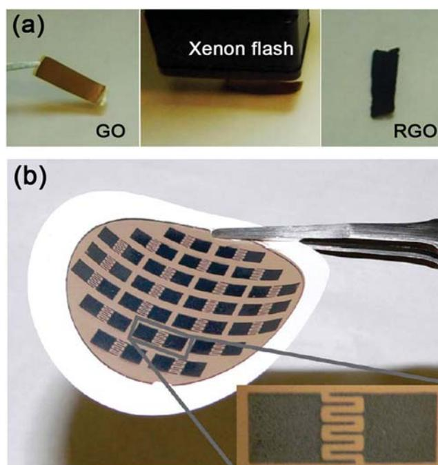
**Figure 2.** Flash reduction of GO. a) Photographs of GO, flash reduction of GO and RGO, from left to right; b) photograph of the arrays of RGO/polystyrene interdigitated electrodes fabricated on a 1.5 inch diameter GO/polystyrene thin film deposited on a Nylon filter paper. The inset shows the close up view of one set of such electrode. Reproduced with permission.<sup>[81]</sup> Copyright 2008, American Chemical Society.
