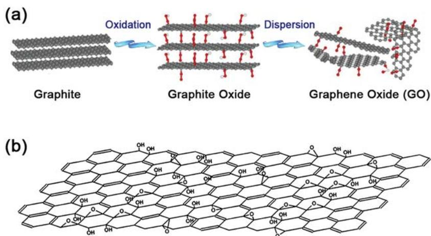
**Figure 1.** a) Schematic illustration of the preparation of GO from graphite; b) Schematic illustration of the structural model of a GO sheet. Reproduced with permission.<sup>[91]</sup> Copyright 1998, Elsevier.
