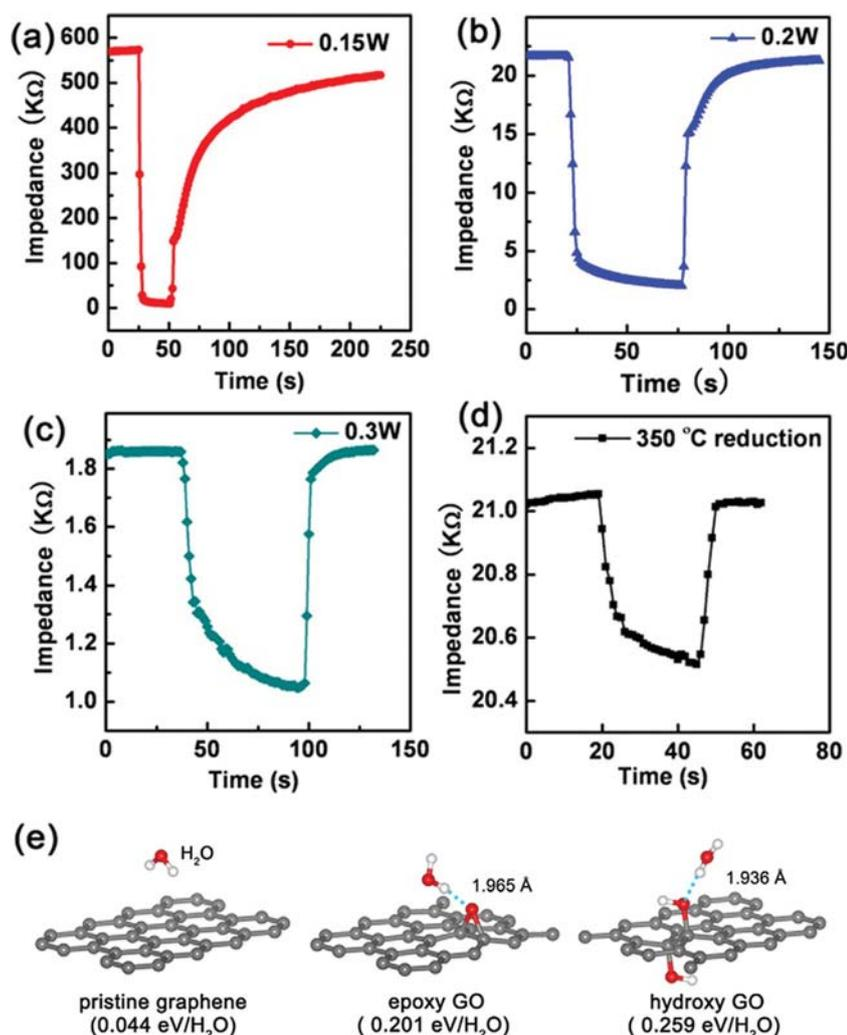
**Figure 10.** Response and recovery properties of the RGO sensor. GO films were reduced under the laser power of a) 0.15 W, b) 0.2 W, and c) 0.3 W; d) GO was also reduced at 350 °C under the protection of nitrogen for comparison. e) Response/recovery curve of RGO (0.2 W) sensing device for five cycles. The curves were measured between 11% and 95% relative humidity at room temperature. Reproduced with permission.<sup>[162]</sup> Copyright 2012, Elsevier.
