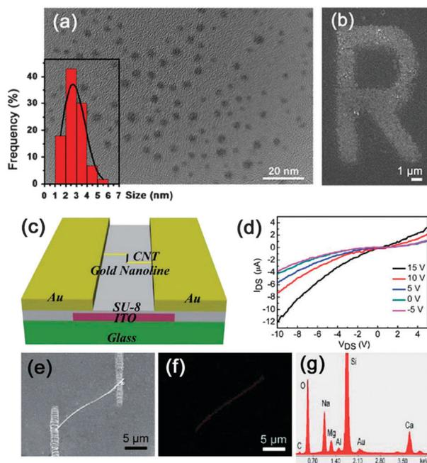
**Fig. 6** (a) Uniform Ag NPs used for FsL-PDA. Inset is the size distribution of the NPs. (b) An "R" letter assembled from Ag NPs. (c) Design for a MWCNT-FET fabricated via FsL-PDA. (d) Output characteristics and (e) SEM image of a MWCNT-FET. (f and g) Energy-dispersive X-ray (EDX) map and spectrum of the MWCNT-FET in (e). (Reproduced from ref. 111 and 112 with the permission of IOPscience and the Royal Society of Chemistry.)
