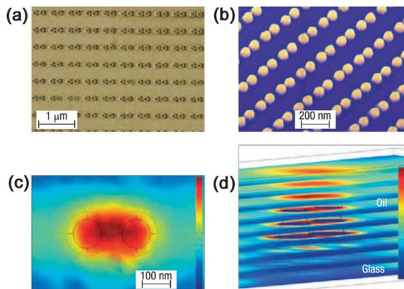
Fig. 4 Electron micrographs of an array of nanopillar pairs, (a) overlook and (b) under a tilted angle. Every nanopillar was 90 nm in height. (c) Optical field intensity distribution of a plane about 200 nm above the substrate. (d) Different planes of optical field intensity distributions of a nanopillar pair, separated by 50 nm. (Reproduced from ref. 104 with the permission of the Nature Publishing Group.)
