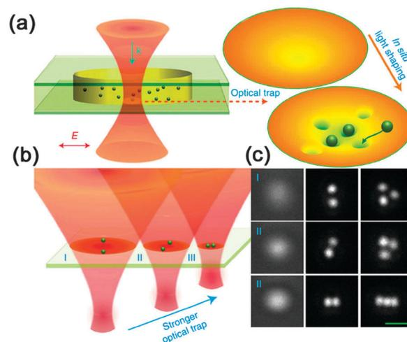
Fig. 2 (a) Cooperating optical trapping and optical bonding for assembling arrays of NPs. (b) The trapping planes could be chosen by modulating the position of the focus. (c) Optical images of single, double and triple Ag NPs (100 nm) trapped in the different planes illustrated in (b). Scale bar is 1  $\mu\text{m}$ . (Reproduced from ref. 85 with the permission of the Nature Publishing Group.)
