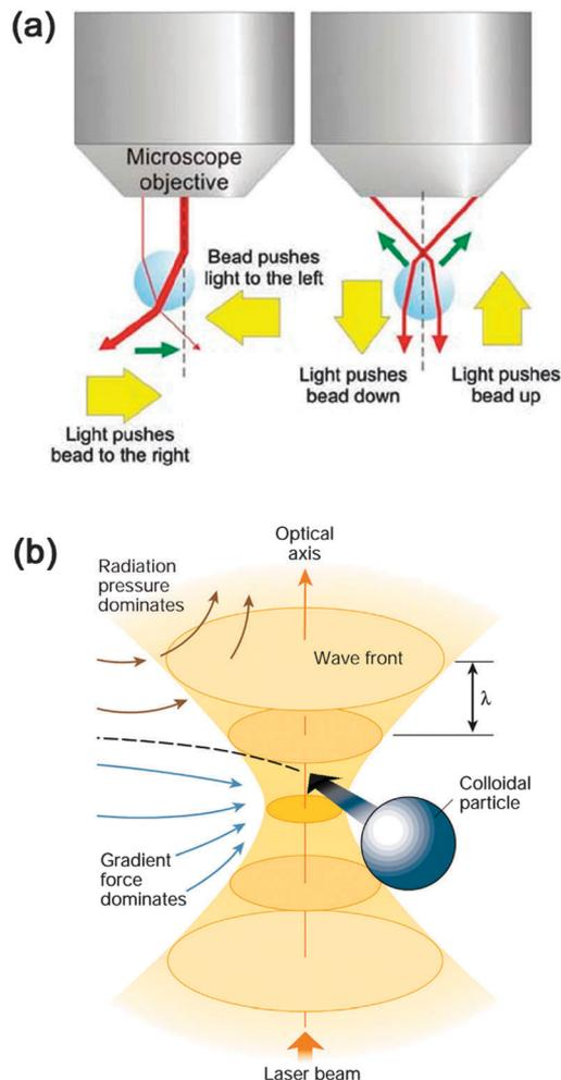
Fig. 1 Schematic illustration of the basic principles of OT: NPs at (a) a geometric optical size and (b) a Rayleigh size. (Reproduced from ref. 72 and 73 with the permission of Elsevier and the Nature Publishing Group.)
