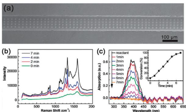
**Fig. 8** (a) A microchannel fully assembled with Ag clusters. (b) Raman spectra collected during the catalysis reaction. (c) Micro-region absorption spectra of the microfluids during the catalysis reaction. The inset of (c) is the kinetic study of the reaction. (Reproduced from ref. 123 with the permission of the Royal Society of Chemistry.)
