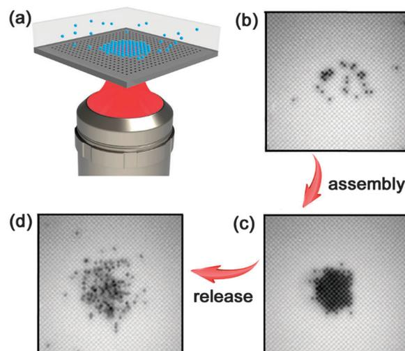
Fig. 3 (a) The principle of resonant cavity aid assembly of 520 nm colloidal particles. (b–d) The process for the assembly and release of the particles by modulating the resonance of the microcavity. (Reproduced from ref. 102 with the permission of the American Chemical Society.)
