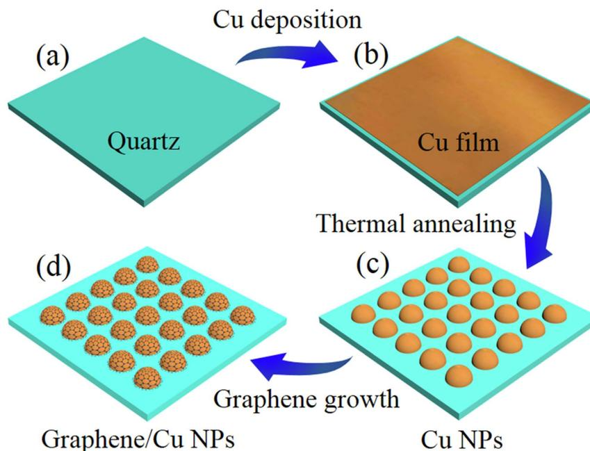
**Figure 1.** Schematic illustrations of fabrication sequences for the as-grown graphene/Cu NPs hybrid nanostructures. (a,b) Deposition of the Cu film on the quartz substrate. (c) Thermal annealing of the Cu film. (d) Deposition of the graphene on the Cu NPs.
