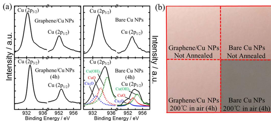
**Figure 7.** Time evolution of the XPS core-level Cu2p spectra (a) and photograph images (b) of graphene/Cu NPs hybrid nanostructures and bare Cu NPs before and after thermal treatment at 200°C for 4 hours.
