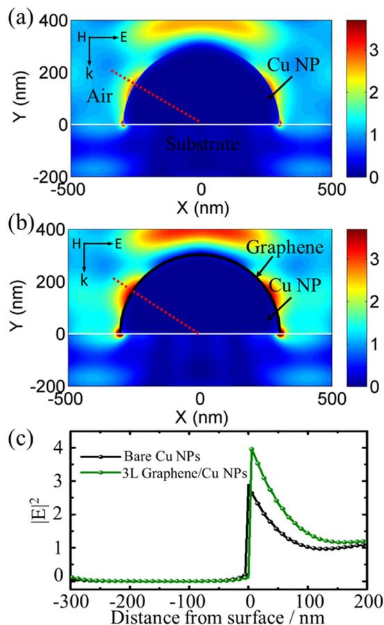
**Figure 4.** Simulated electrical field distributions for the bare Cu NP (a) and as-grown graphene/Cu NP hybrid nanostructure (b). (c) Cross-section plots for total electric fields of Cu NP along the red dot line in (a,b) with (green) and without (black) graphene layer, respectively.
