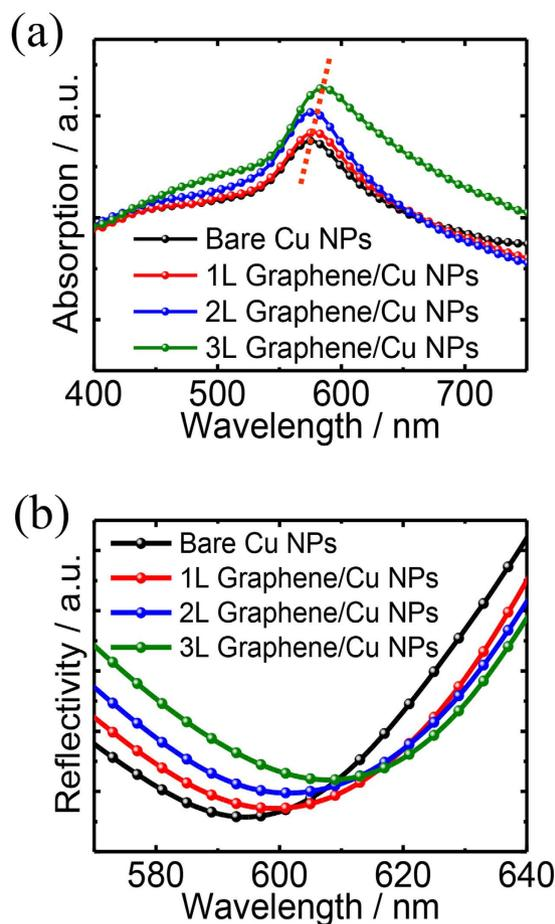
**Figure 3.** (a) Steady-state optical absorption spectra versus wavelength for the Cu NPs coated with various numbers of graphene layers. (b) Simulated reflection spectra of Cu NPs coated with various numbers of graphene layers.
