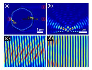
**Fig. 5.** Optical intensity distribution of pierced microdisk based on FDTD simulation. (a) The global intensity distribution. The light scattering occurs at the hole position and the light emission forms in the direction of 0 deg. The definition of the initial angle is the same as Fig. 4(b). (b)–(d) the enlarged detail graphs of regions 1, 2, and 3 in (a).
