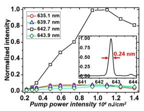
**Fig. 3.** Measured intensity of output light varies with the power of the pump laser. The light with a wavelength of 642.7 nm is amplified and shows the lasing property. However, the other light, with wavelengths of 635.1, 639.7, and 643.9 nm, cannot be amplified. The inset shows the spectrum enlargement at a wavelength of 642.7 nm with pump power intensity of  $1.1 \times 10^4$  nJ/cm<sup>2</sup>.
