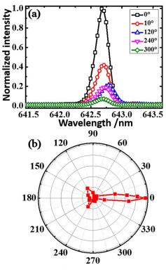
**Fig. 4.** Characterization of the directional emission property of the pierced microdisk. (a) The emission spectrum of the pierced microdisk at different detection angles. (b) The relationship of lasing intensity distribution with detection angles at a wavelength of 642.7 nm. The definition of the initial angle is the same as Fig. 5(a).
