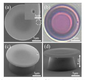
**Fig. 1.** Geometric morphology of the pierced microdisk. (a) The top view scanning electron microscopy (SEM) image. The inset shows the local amplification image of the microdisk. (b) The optical microscope photograph of the pierced microdisk. The center region with deeper color is the cone-shape pedestal shown in Fig. 1(d). (c)–(d) The 45 deg tiled view and the side view of the microdisk SEM image.
