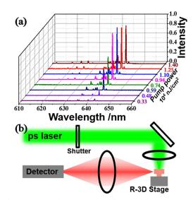
Fig. 2. (a) Normalized 3D-waterfall arranged emission spectrum from a 20- $\mu$ m-diameter pierced microdisk pumped with increasing power intensities of 532 nm picosecond laser. (b) The schematic diagram of excitation and collection system. The microdisk was placed on a R-3D stage composed of a rotary stage and a 3D displacement platform.
