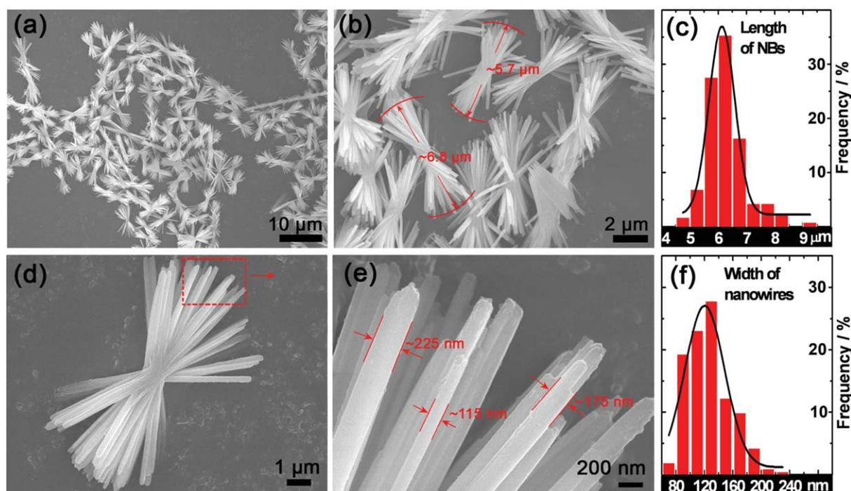
**Fig. 1** a and b) SEM images of CdTe NBs; c) statistical analysis of the length of NBs; this length distribution was calculated based on two hundred NBs; d) an SEM image of one typical CdTe nanobundle; e) a magnified SEM image of one side of a NB; f) statistical analysis of the width of the nanowires; this width distribution was calculated based on five hundred nanowires.
