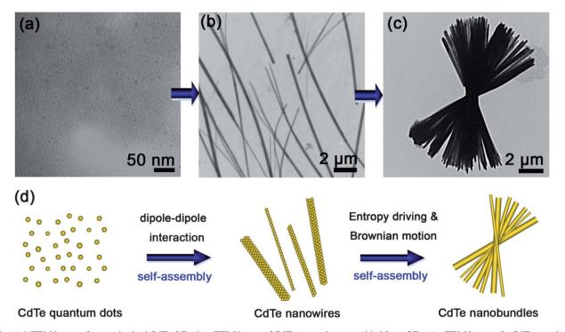
**Fig. 2** a) A TEM image of as-synthesized CdTe QDs; b) a TEM image of CdTe nanowires assembled from QDs; c) a TEM image of a CdTe nanobundle assembled from nanowires; d) a scheme for the hierarchical assembly of CdTe QDs into nanobundles.
