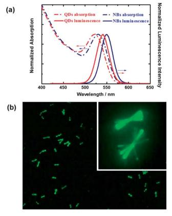
**Fig. 4** a) Absorption (blue and red dash dots) and luminescence spectra (blue and red solid lines) of CdTe QDs (red lines) and NBs (blue lines). A 10 nm red-shift was observed in both the absorption and luminescence spectra of NBs compared with pristine QDs; b) a luminescence microscopic image of the CdTe NBs, inset is the magnified image of two NBs.
