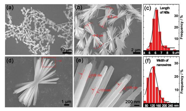
**Fig. 1** a and b) SEM images of CdTe NBs; c) statistical analysis of the length of NBs; this length distribution was calculated based on two hundred NBs; d) an SEM image of one typical CdTe nanobundle; e) a magnified SEM image of one side of a NB; f) statistical analysis of the width of the nanowires; this width distribution was calculated based on five hundred nanowires.
