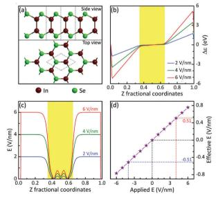
**Fig. 1** (a) A schematic diagram of an InSe monolayer. Color coding: dark brown for In; and green for Se. (b) Potential energy differences ( $\Delta e$ ) induced by electric fields along the Z direction. (c) Electric field intensity distribution along the Z direction (vertical to the plane). The region shaded in yellow indicates the thickness of the InSe monolayer. (d) The effective electric field intensity (effective E) in the InSe region as a function of the applied value (applied E).
