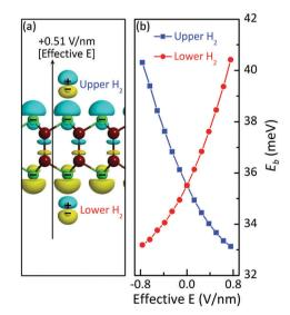
**Fig. 5** (a) Charge density difference distribution in InSe with two H<sub>2</sub> molecules adsorbed, under a +0.51 V nm<sup>-1</sup> effective field. Atom and CDD isosurface color coding is the same as in Fig. 3. (b) The binding energy ( $E_b$ ) for the upper H<sub>2</sub> (blue line) and lower H<sub>2</sub> (red line) on InSe surfaces *versus* the effective field.
