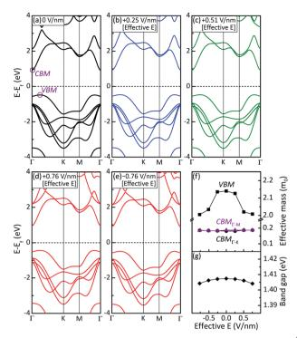
**Fig. 4** The band structures of an InSe monolayer under (a) 0 V nm<sup>-1</sup>, (b) +0.25 V nm<sup>-1</sup>, (c) +0.51 V nm<sup>-1</sup>, (d) +0.76 V nm<sup>-1</sup> and (e) -0.76 V nm<sup>-1</sup> effective electric fields. (f) The effective masses at the VBM (holes) and CBM (electrons, along the  $\Gamma$ -K and  $\Gamma$ -M directions) and (g) band gap versus the effective electric field.  $m_0$  stands for the electron rest mass.
