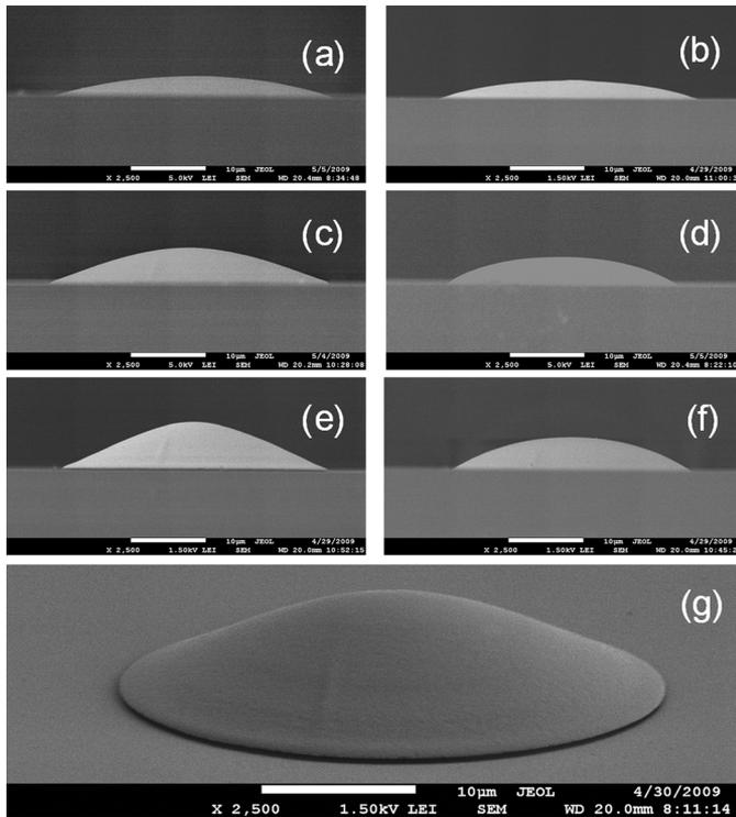
Fig. 2. Logarithmic axicons with different pairs of  $d_1$  and  $d_2$ . (a), (c) and (e) are lateral views of FLAs; (b), (d), (f) are of BLAs. (g) is a skew view of (c).
