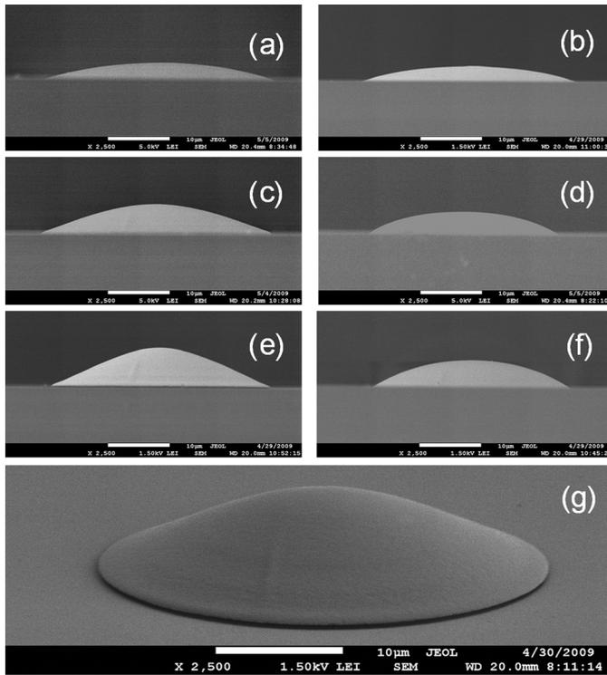
Fig. 2. Logarithmic axicons with different pairs of  $d_1$  and  $d_2$ . (a), (c) and (e) are lateral views of FLAs; (b), (d), (f) are of BLAs. (g) is a skew view of (e).
