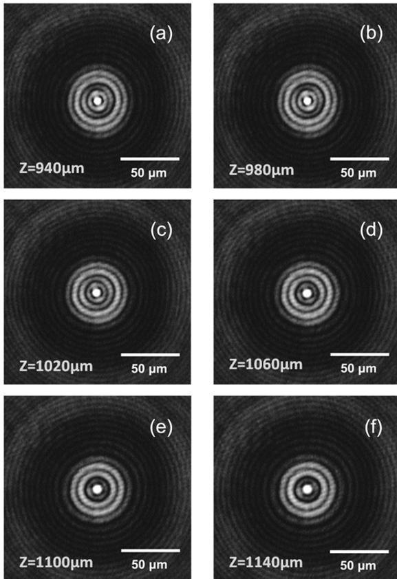
Fig. 4. Approximate Bessel distribution on different cross sections.
