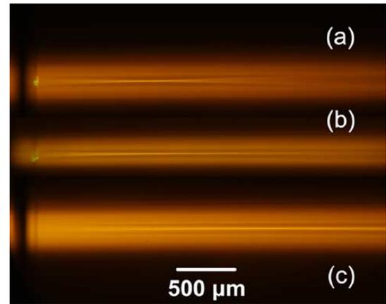
Fig. 3. Lateral view of focal line segments with different lengths.
