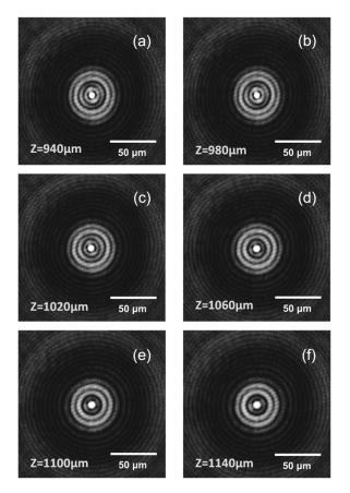
Fig. 4. Approximate Bessel distribution on different cross sections.
