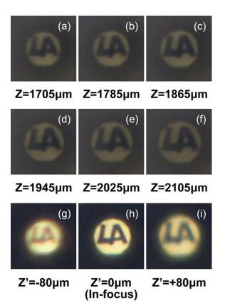
Fig. 5. (a)–(f) Images formed by a logarithmic axicon along the optical axis and (g)–(i) those formed by a common lens.
