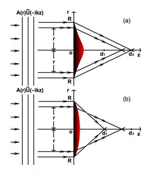
Fig. 1. (a) Forward logarithmic axicon and (b) backward logarithmic axicon.
