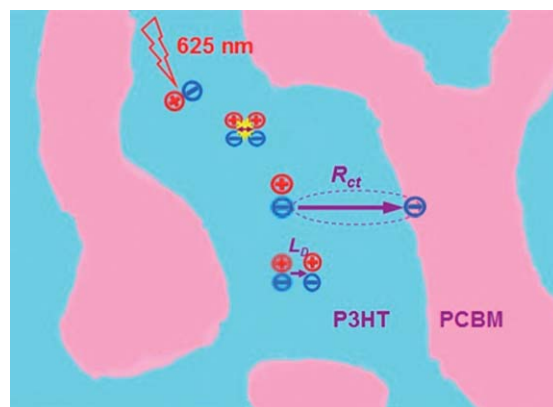
Scheme 1 Illustration of exciton generation, diffusion, annihilation and charge transfer dynamics in nano phase-separated P3HT/PCBM blend films. L_D is the diffusion length in a certain time, R_{CT} is the charge transfer radius.
