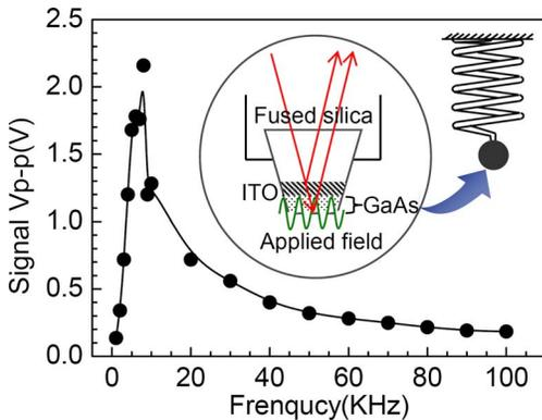
Fig. 2. (Color online) Response of the GaAs film probe to the excitation by an external electric field at low frequency. The inset is an illustration of the probe with the thin GaAs layer fixed to the base on the upper end, while the lower part is freely movable. The oscillation of the GaAs layer is therefore considered equivalent to a simple spring system loaded with its deadweight.
