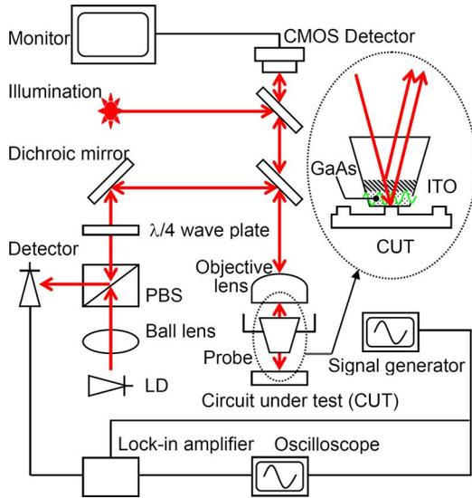
Fig. 1. (Color online) Schematic diagram of the setup for the local electric field detection, where PBS denotes polarization beam splitter. The  $\lambda/4$  wave plate is  $45^\circ$  oriented with respect to the plane of polarization of the incident probing beam.
