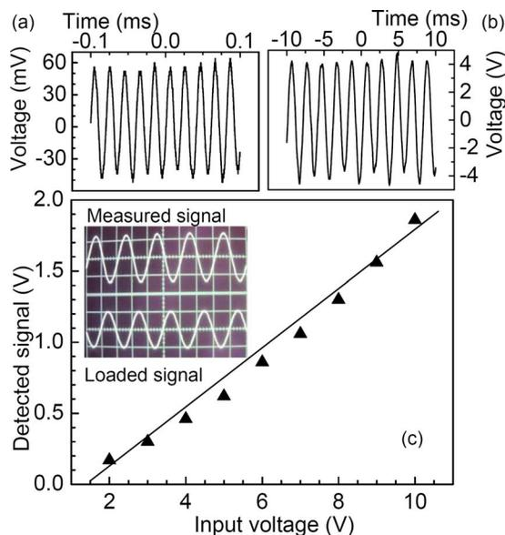
Fig. 4. (Color online) Detection of the electric field above a circuit by a GaAs probe. Waveforms measured at (a) high-frequency (50 kHz) and (b) low-frequency (0.5 kHz) fields. (c) Relation between the signals collected and the voltages applied to the circuit. The inset is a typical oscilloscope screen.
