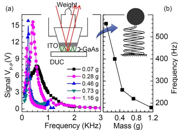
Fig. 3. (Color online) Resonant frequency of the GaAs thin film versus loading weights of 0.07, 0.28, 0.46, 0.73, and 1.16 g. (a) Responsive spectra and (b) loading-weight-dependent resonant peak wavelengths. Oscillation of the film is similar to the case of Fig. 2 but with an increased loading (the weight of the silica base and metal rings).
