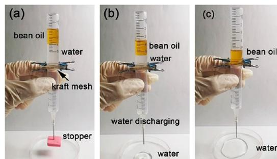
**Figure 8.** Gravity-induced oil–water separation based on the kraft mesh. The kraft mesh with a 100  $\mu\text{m}$  hole size/200  $\mu\text{m}$  hole distance was sandwiched between two plastic tubes.
